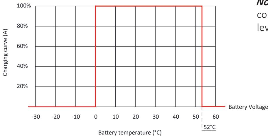
**Notice:** No temperature compensation on voltage level when setting LiFePO4
